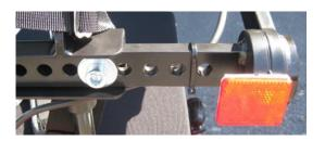
Untighten the two screws. Now you can adjust the armrests in the width. If you have adjusted them to the desired width, tighten the screws.
