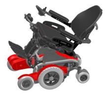
With the option "Tilt in space" it's possible to tilt the seat to an angle of approx. 30° to the back, this leads to a more comfortable seat-/ rest-position. The "Tilt in space" is a good prevention against decubitus by the way.
