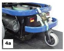
• Lift the back wheel up with a clamping set.
